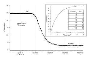
This diagram shows a typical pattern of a phase change from beer to water, which takes place within about 20 seconds. The PhaseGuard C picks up this interface change quickly and with high precision. It allows the user to select the switching point which he believes is the optimum (compromise between beer loss or amount of water in the storage tank).
